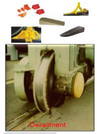
There have been over 15 accidents and near misses reported involving cranes that have traveled too close to, into, onto, or over chocks and wedges (wooden and metal). These events occurred during all phases of work, including the repositioning/stowage of cranes, during operator daily checks, and during production and maintenance evolutions.
